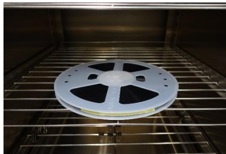
Figure 5. Example for Baking the LEDs
